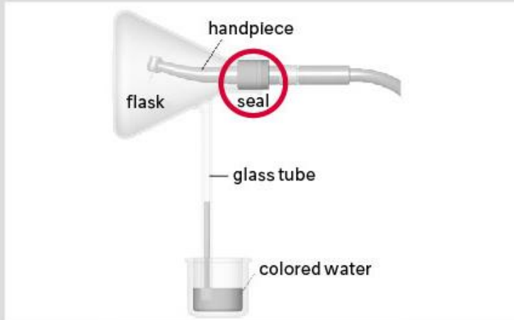
Fig. 1 Complete test setup : Measuring suckback pressure of the whole handpiece brand.
