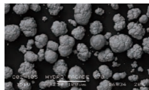
FLASHpearl (calcium carbonate) Average particle diameter: 54µm Scanning electron microscope image magnification of 150X
